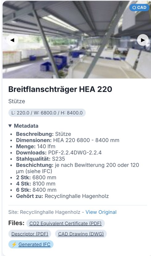
Figure 3: A single card element of a reclaimed component with extracted metadata, cost, CO 2 , and access to Building Information Modelling (BIM)-ready exports. It is readily available for drag-and-drop into the workspace and suitable Computer-Aided Design (CAD) software. Multiple media items can be uploaded and attached, also images. Photograph from [1].
